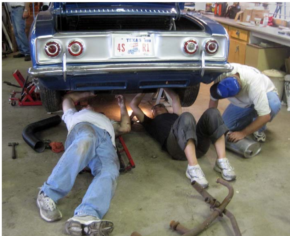
The July 2012 FlatSix Journal covered the activities at Juna Tuna 10. This photo captured Ned Madsen, Christine W. (Monza Gal) and Richard Law checking off repairs: exhaust, heater hose, temp switch. They were working on Christine's LM AC coupe.
