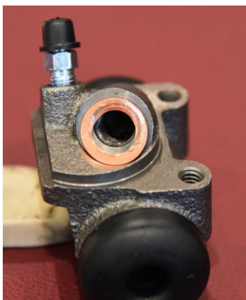
Original GM copper washer; note offset
