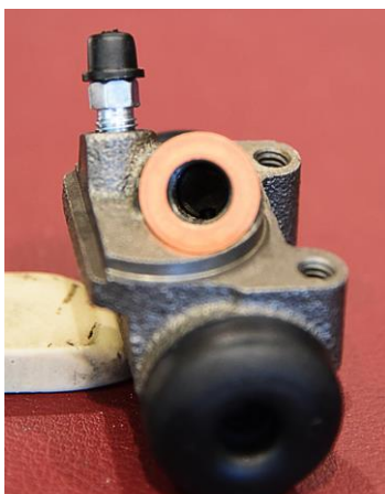
NAPA copper washer; note fit on brake cylinder
