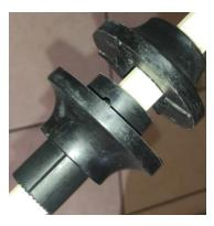
Here's a pair of Bushings ready to be compressed. Don't forget to put some Grease inside that Limiting Compression Metal tube as it could Rust inside. Just remember to bring along a bottle Jack when you change out the Bushings on the 'Lower Control Arm' on your CORVAIR. *Fran*
