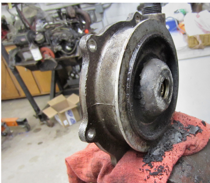
Alex Moats has been working on a 1964 Spyder engine for Lloyd Folger. One of the issues was the turbo was froze. This pile of carbon was a problem.
