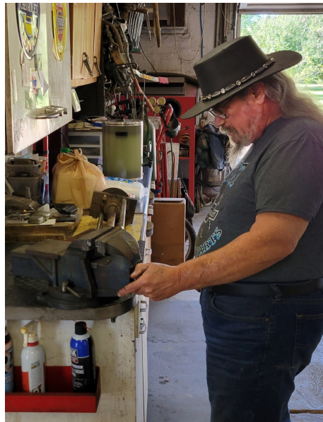
At the 2021 Luna Tuna Dennis Fuller presses the bearing of an EM rear axle. The bearing had failed on the trip to Little Rock, AR for the Corvair Roundup.
