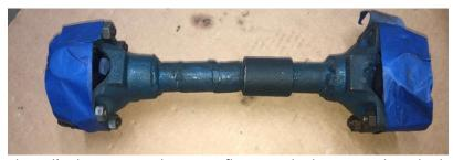
This is the Special Axle I was working on when I tried to use the wrong nut. Using such an axle between the existing axles on a CORVAIR with its engine removed – orients the rear wheels toward each other -this allows pushing the vehicle around the garage or grounds – (NOT on the
