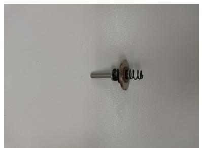
This is the plunger rod that is shorter. It is aluminum and too small for my welder or I would have attached a bead to it and dressed it up. The case is also slightly longer,
