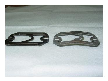
This picture shows a bent retainer that still allowed the rotor and cap to be installed and the engine to run (but not properly).
