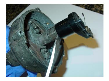
The **wrong** approach to a stuck rotor is to pry up at this point; the **correct** method would be to twist the screwdriver to separate the rotor from the cam. Or you could simply break the rotor off sideways with pliers.
