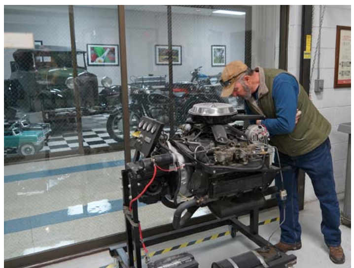
Lee Olsen checks out a 140hp Corvair engine donated by Chris Shade and used to teach tune-up and multiple carburetor synchronization techniques.
