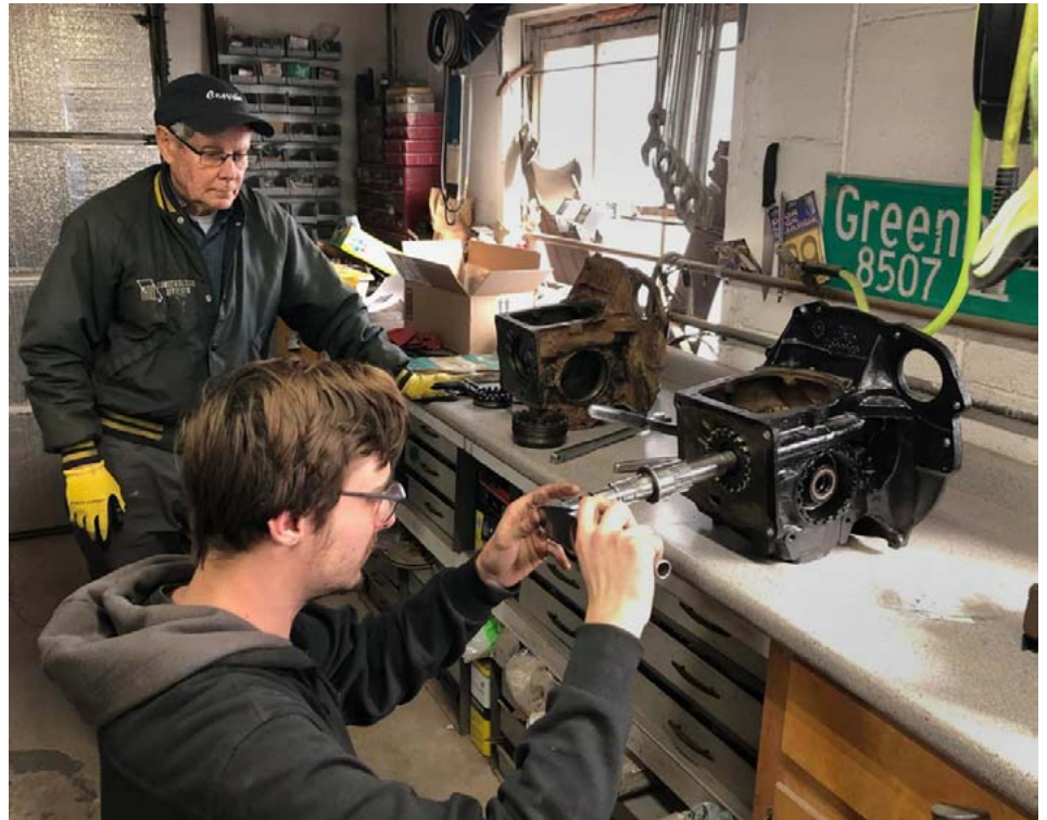
Mike Dawson schools McPherson College Restoration program students and setting up and adjusting a Corvair differential. Sean Whetstone is shown checking the pinion preload with an inch-pound torque wrench. Mark Welte Photo.
