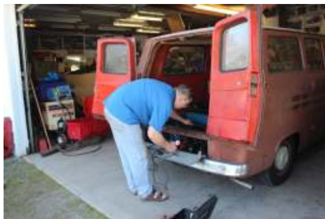
Eric setting the carb s and timing on his frexhly re-built 110 motor on his van.
