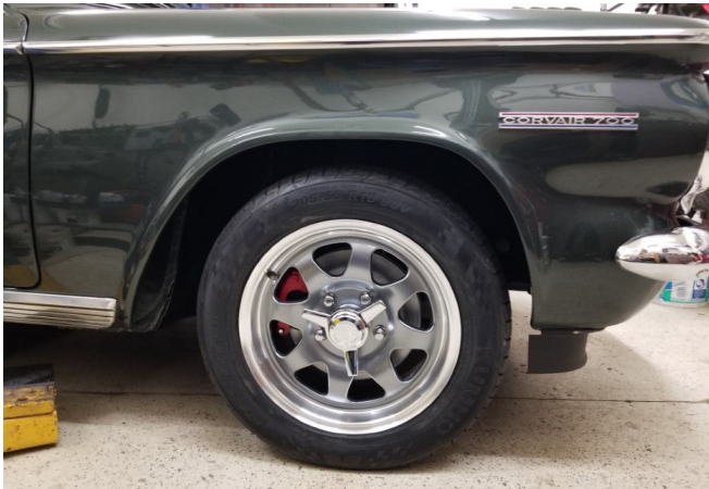
Note conversion from 4 lug to 5 lug wheels on Tom's wagon.
