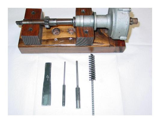
Pictured below is the minimum disassembly necessary to replace the bushing in a '62-'69 ('60-'61 will be similar). This would obviously be the time to also check and lube the advance mechanism.
