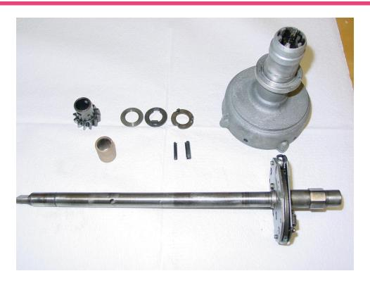
File off any sharp edges at the two pinholes and polish the shaft before fitting the bushing. During reassembly remember the divet on the gear must align with the direction of the rotor notch.
