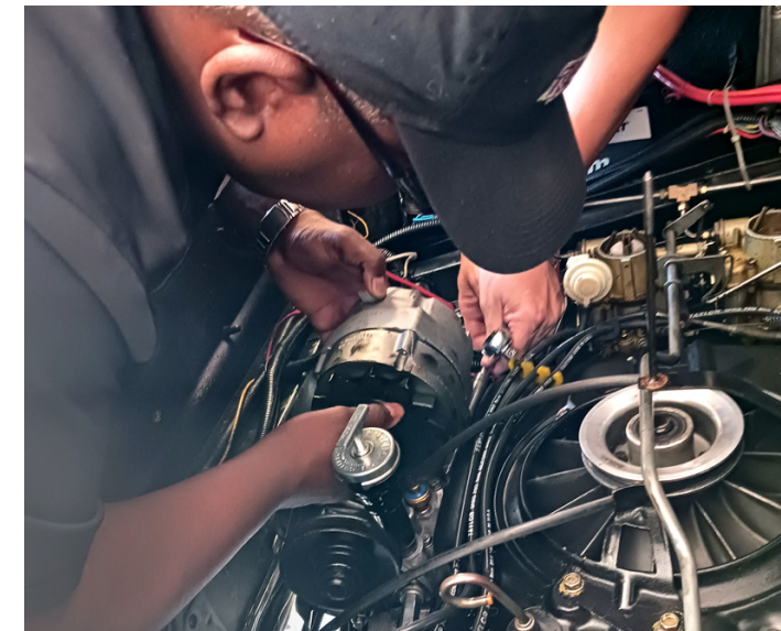
Marcus Trotter helps Brad Stauffer install the alternator on his '68 convertible at the HACOIA tech day.
