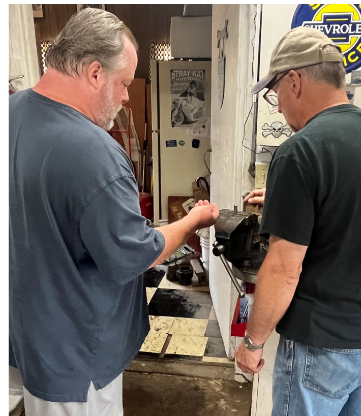
Eric Kline and Mark set up the bucking die to install the stainless steel rivets that hold the ignition wire separators to the top shroud. Mark used the setup on his chrome top shroud. Bill Smith photo.
