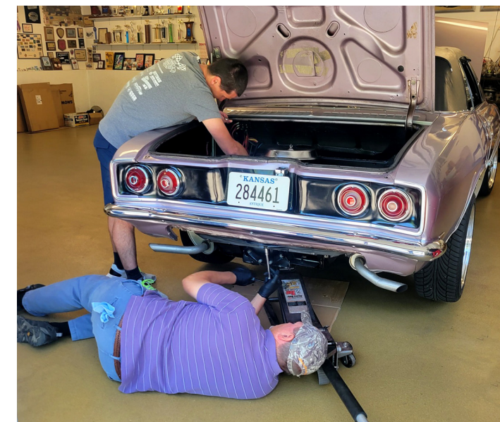
Chris Green and Brad Stauffer work as a team to replace a failed rear engine mount at the tech day.
