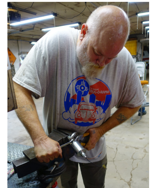
Bill Smith worked on fuel issues on Tiffany's '64. He replaced the filter and rerouted lines on the electric pump and replaced a leaking fuel tank sending unit.
