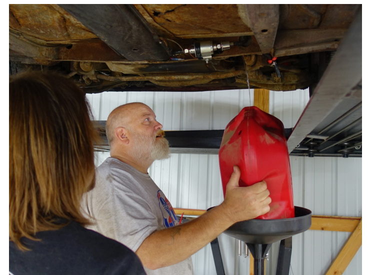
Bill Smith worked on fuel issues on Tiffany's '64. He replaced the filter and rerouted lines on the electric pump and replaced a leaking fuel tank sending unit.
