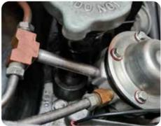
After installing the pump and wiring incl. Crash emergency stop (the fuel pump will be switched off in the event of a collision) everything works perfectly again for the time being.
