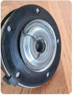
I replaced the diaphragm plate with a dummy, so that I could reinstall the original fuel pump and the fuel supply line and the lines to the carburettors as well.
