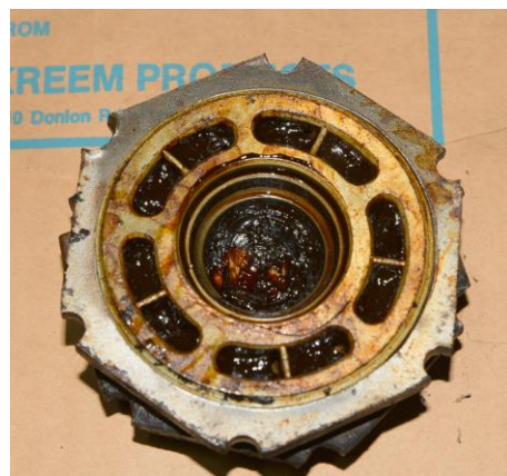
Worm Gear Adjusting Nut and Bearing Race
