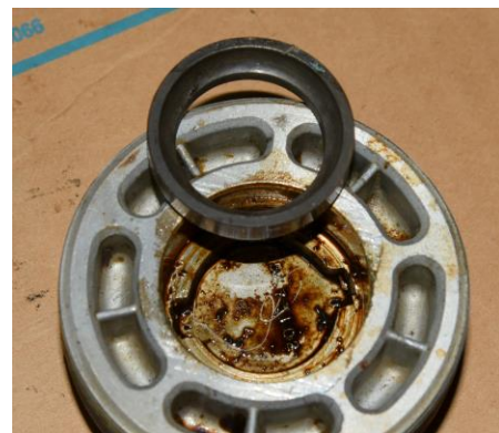
Race Removed, Note the Two Recesses
