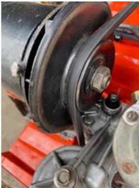
This is how the belt and pulley are designed to fit
