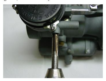
Cut off the threaded part of the casting at the end of the threads and drill the hole to 9/32". Then follow up with a 5/16-24 tap. Carefully clean out chips that could freeze up the choke piston.
