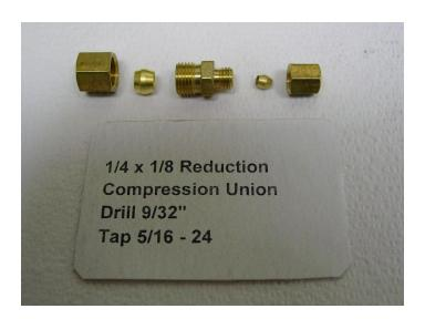
This is a brass fitting assembly that you can use just the union body to replace the bad casting that you removed. The small end threads into the newly created threaded hole and the large end has the same threads and size as the choke heat tube. Order the part with the exact two line nomenclature above.
