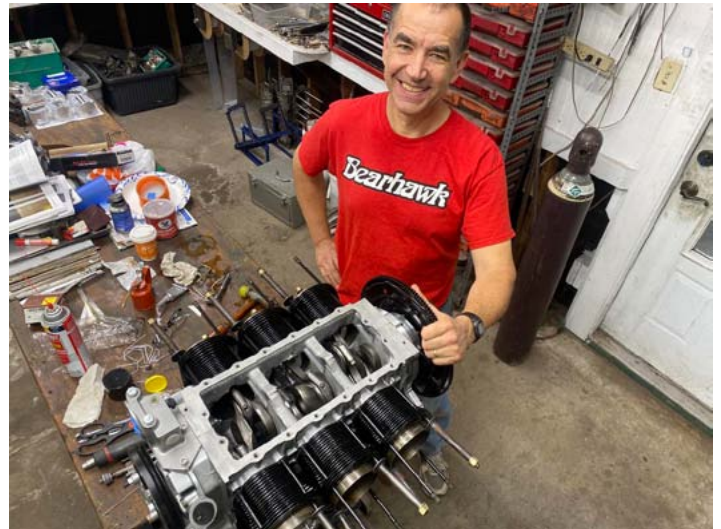
David and his 3.3 in progress. The stroked Corvair engine comes with added expense. They require more patience and dexterity to assemble, but not an obstacle for David, and the smile tells the story
