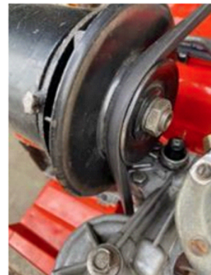
This is how the belt and pulley are designed to fit
