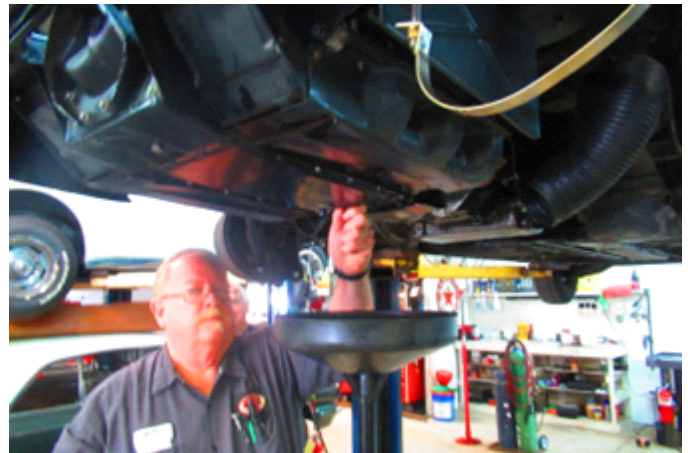
Jeff's draining the oil pan in prep for separating the bell housing from the engine.
