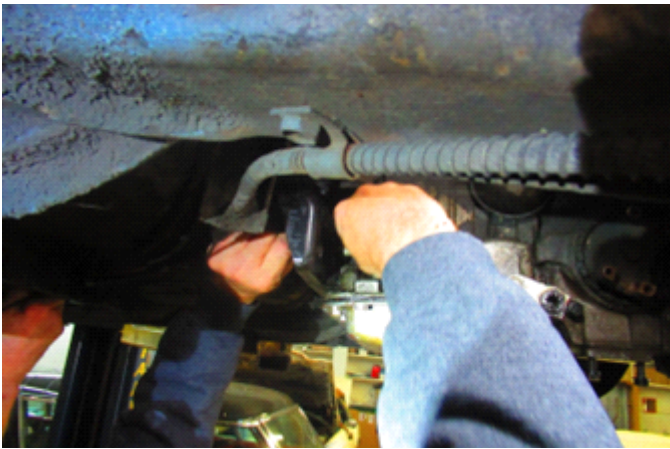
Larry Asheuer demonstrates the technique for disconnecting the shift cable from the transmission. Twist and separate!
