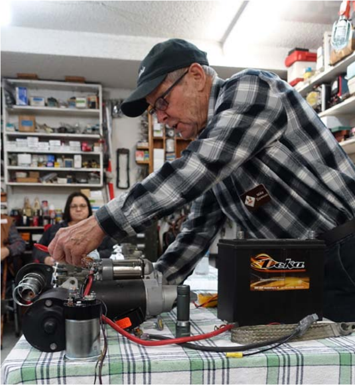
At the HACOIA Tech Session, Mike Dawson explains how to use a multi-meter to diagnose starter issues.
