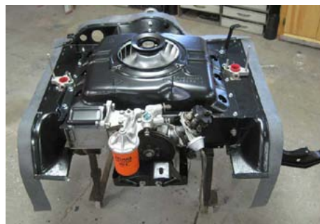
LEFT Since the powerpack had to be pulled to replace the faulty flywheel Terry took the opportunity to clean the engine and add new seals.
