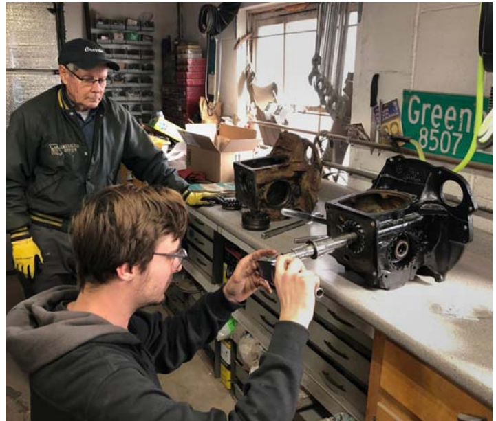
At the 2023 Cold Tuna, Mike Dawson schools McPherson College Restoration program students and setting up and adjusting a Corvair differential. Sean Whetstone is shown checking the pinion pre-load with an inch-pound torque wrench. Mark Welte Photo.
