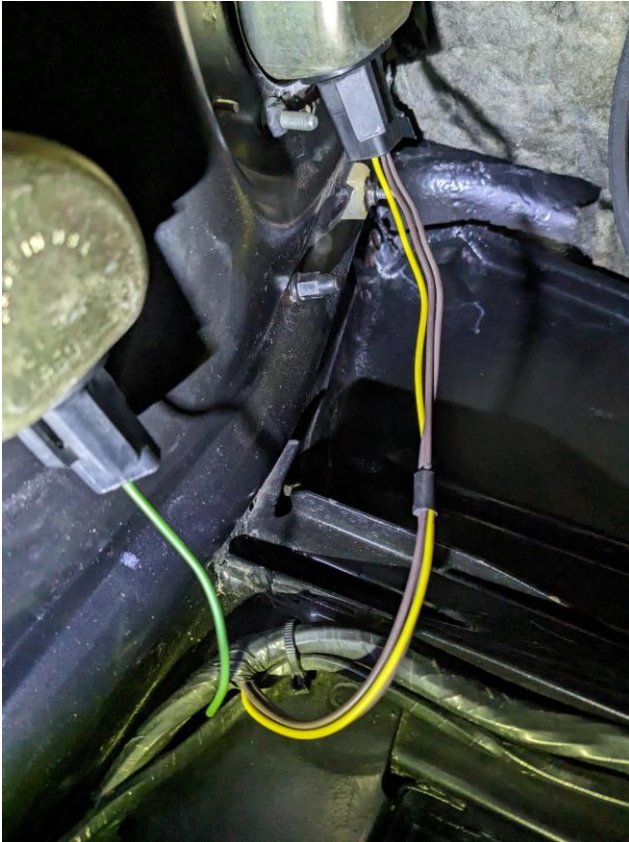
Left Brake/Turn/Parking Light. This is a reproduction harness; Note the pair of brown wires and the single solid yellow wire.
