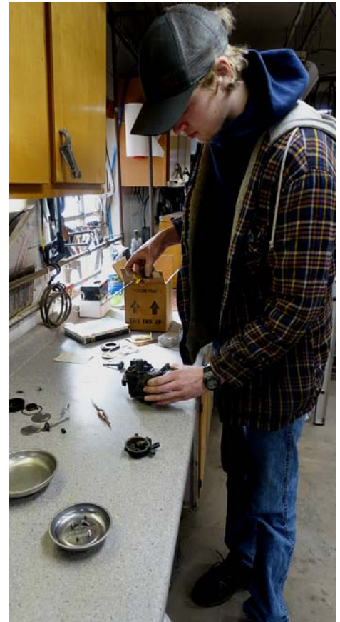
Edwin Butier worked on a turbo carburetor. This one had been bored out to flow more air..
