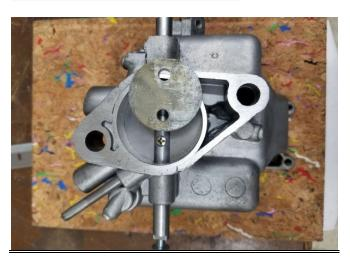
I still have to drill out the passages for the vacuum tubes in the base and do a few other small modifications.
