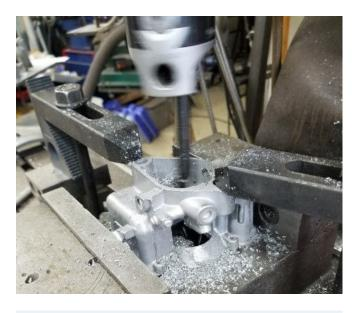
Then the sleeves were jb welded in along with filling the area of the cluster that I will eventually smooth and bevel to help airflow. I then bored it out to exactly 1.500".
