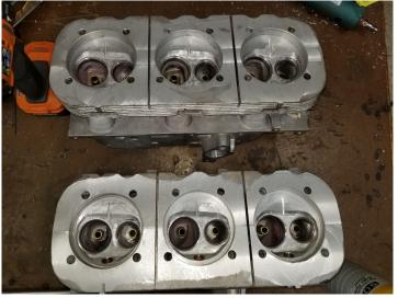
The Compression Ratio is 9.5:1 with a .042 head gasket and the step milled out. I am running 2 "carb" bases so I welded the secondarys shut so I can use the stock sheet metal.
