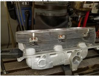
I also opened up the remaining opening to 1.5" because that will be the size of the "carb" throttle body plate. Since the motor in the car is already a Ted Brown FI system, I am making my own replacement bases that will flow more air. I am basing these mods on the Yenko carburetor mods. In a discussion with Bob Coffin he mentioned that Yenko used the throttle plates from the turbo carbs and sleeved the throat.
