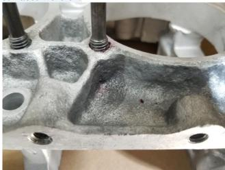
Here are 4 of the studs from the case that fortunately I was able to remove with using heat and Kroil. I have taken apart several engines and save the good studs. I used these as replacements and they tightened down nicely, also added loctite to make sure no oil leaks.
