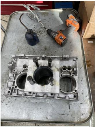
Then washed thoroughly in hot dawn dish soap and rinsed, blown dry and then used heat gun to drive off all moisture. Then did white cloth test and no residue.
