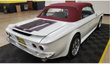
1963 Corvair Monza Convertible Restomod - 383 Stroker V8 Fitted onto a C4 Corvette chassis - 700R4 auto transmission with overdrive
