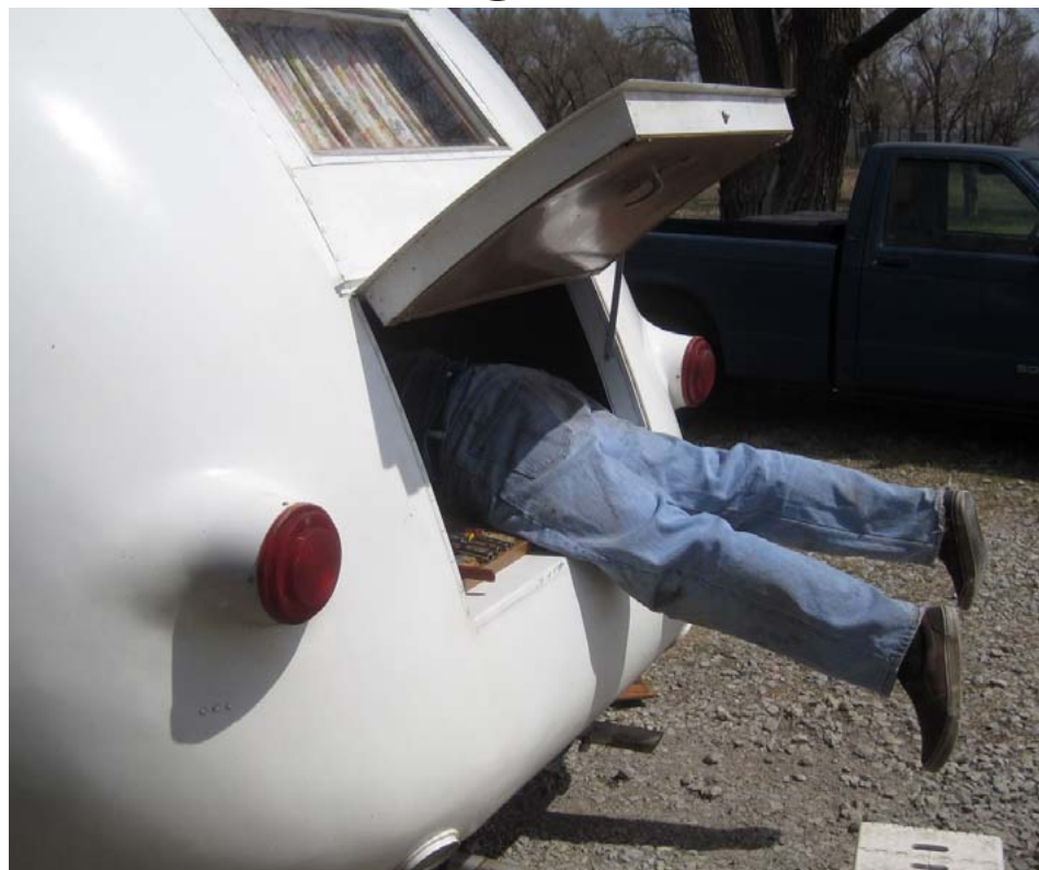
Ten years ago Ned Madsen was really getting into helping Owen Strawn pull a head on Owen's Ultra Van. The Van dropped a valve seat on the trip from Florida. There is about 3 feet of floor before the engine compartment, which makes working from the rear awkward.
