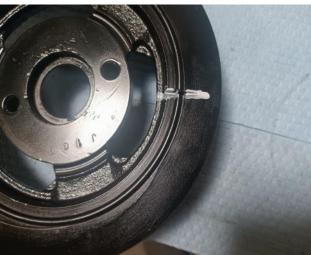
The picture of the fresh balancer shows where I used a white Sharpy to highlight the hash mark and also the timing notch on the outer edge of the pulley.
