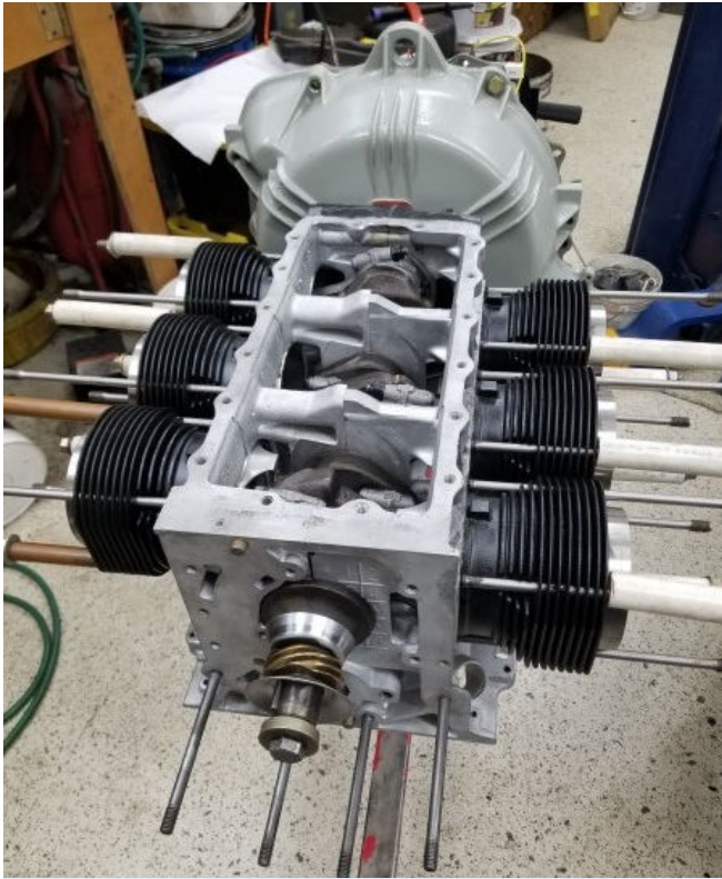
All Cylinders installed and clearances look good. Next up are baffles!!!!!! Don't want to forget.
