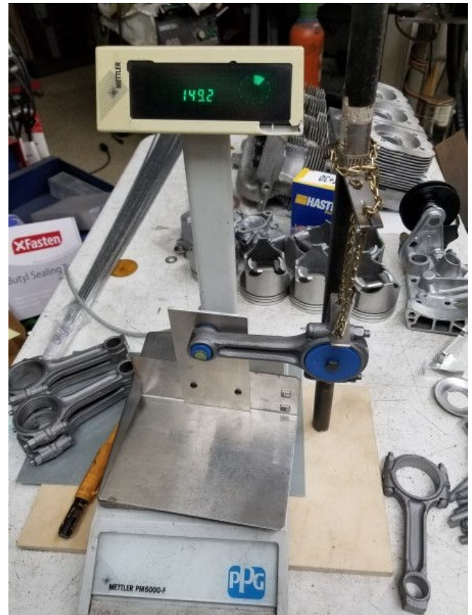
Balanced small and large end of rods.
