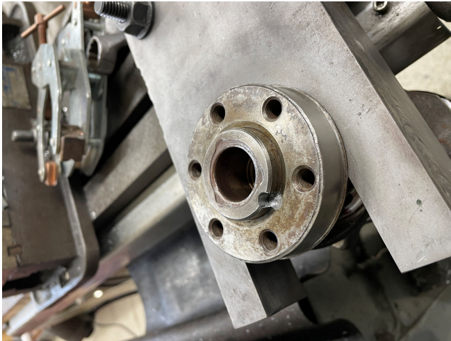
Drilled and tapped cam gear and pinned crank gear for piece of mind.
