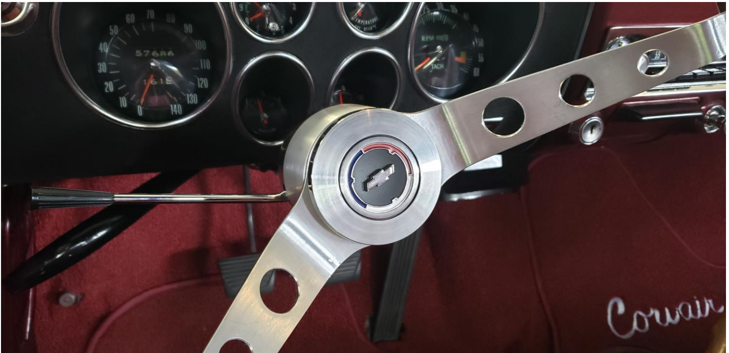
With the steering box centered, the steering wheel was off this amount.
