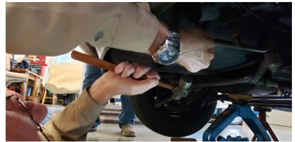
Using a small hammer to loosen the lock nut – we also needed a big hammer. That lock nut was tight!
