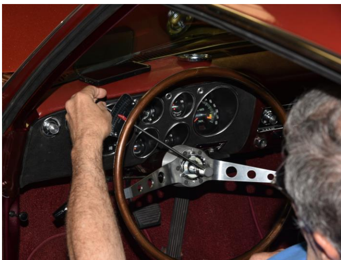
Bill Hubbell checking steering box torque.
