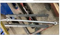
When installing Seth Emerson's bump steer kit Dan had to use a thread file so the new sleeve would accept those old inner tie rods. While everything was apart, he welded a couple of pieces of angle iron to the steering linkage and added a nylon bushing for the pitman arm. Left and below left. Thanks for the update Dan!
