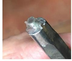
worked to snip away at the end of that 5//16" Allen till I had a short – Fat – square ended blade aimed right across the hole I had made. It has to be centered as the hole in the Jet is exactly in the center and that lines up perfectly with the slot for the blade of the Tool. You must have each of these ideas in mind as the carving takes place.
