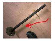
This is a bare FC axle. Splined on one end to accommodate the Axle Yoke (that mates
