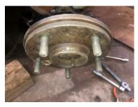
Now, using a single Lug-Bolt, attach the Donor Ring to the back of the 4-Bolt Axle's Flange. You will have to line up the two big holes used for mounting the Wheel Bearing to the A-Frame. You know this single bolt will be placed correctly because you measured the Bolt – Circle (above) and are confident of your measurement! When you have the Donor Ring's remaining four holes behind the four-bolt axle flange you can see where to drill holes to allow the new bolts to come through. You
