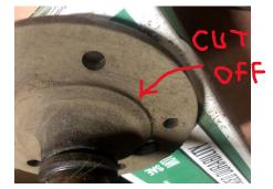
axle flange (outside of the ridge) giving you a ring of flat steel with five holes in it. These holes will hold the new longer Lug-Bolts needed to reach through the 4-Bolt axle's flange to capture the wheel. Sounds kinda weird to say you cut off the holes!
