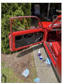
Jason, like most of us, is continually fine-tuning his 1962 Corvair, Flo. In his words this is a "fiddly thing": cleaning up the heat vents and door panels. It seem a PO did a "horrible hack job" installing sound system speakers in the doors, there were no vapor barriers so it was damp and musty in there. He's applied a rust inhibitor at left and is cleaning up the arm rests. Nice work Jason!
