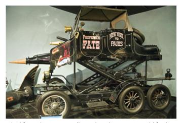
The lift mechanism actually works. That way, it could ford deep streams and rivers on the way to Paris!
