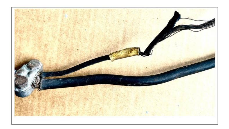
The Batt Cable is for the high current to the starter, right? The little wire on that same terminal feeds ALL other circuits in your CORVAIR. There are a few inches of that wire purposefully made of a smaller gauge wire. Usually you can see the splices where the little wire has been added in.
