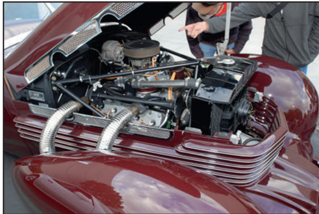
Cord Lycoming V8. Supercharged & side pipes for '37.
