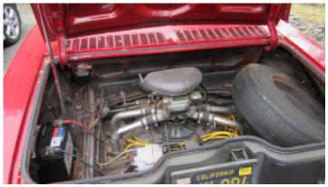
Here is the 140 with a center mount Holly carb. She fired right up (with a new battery) and idled well. A good sign!
