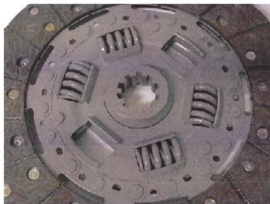
Below is pictured a Vega disc with damper springs and the center splined hub machined to clear the crankshaft hub on a Corvair.
