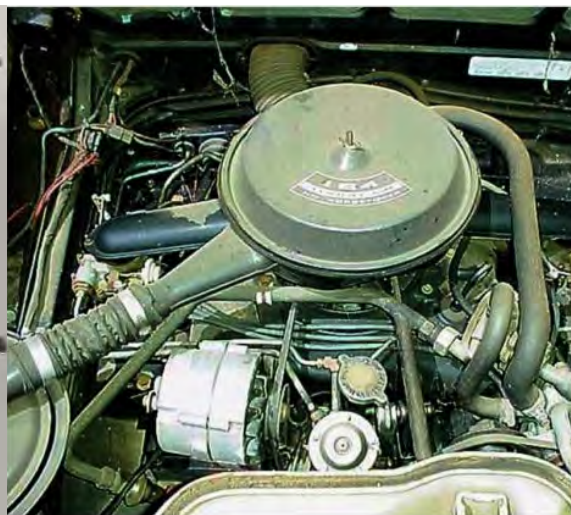
Left: A.I.R. PCV tube - item 5 Above: 2-carb A.I.R. engine with K47 Right: A.I.R. PCV tube
