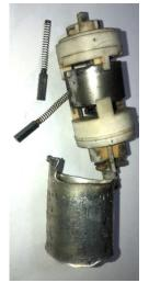
An Electric motor is immersed in the Fuel so that the Fuel can easily be taken into the pump and expelled by use of a hose going out to the gas line. The Pump will never get HOT so long as it is full of the liquid gas. The photo on the left shows the inner pump
