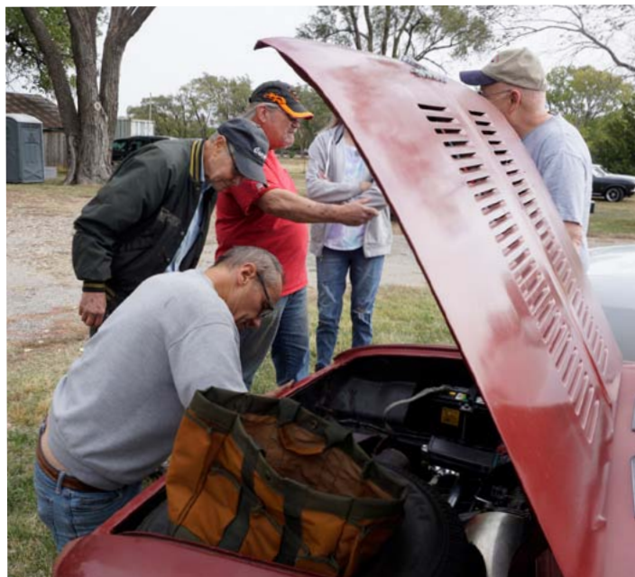
Bob installs the "dummy" pump to replace the leaking manual pump in his Spyder. He already had an electric pump installed in his fuel system.
