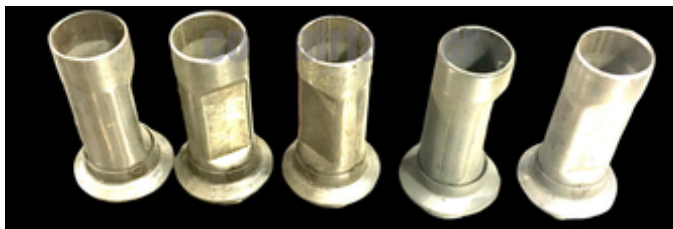
Exhaust tubes press-fit into the bottom of the cylinder heads. One for each cylinder. Five shown here.
