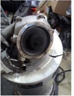
day! Things were improving and that is when Charley noted there was no oil feed line to the turbo. Turbos need a constant supply of oil to keep the bearing inside cool. A Corvair turbo impeller could spool up to 50,000 - 60,000 RPM's. Then we noted that the turbo housing itself had a plug where the line was
