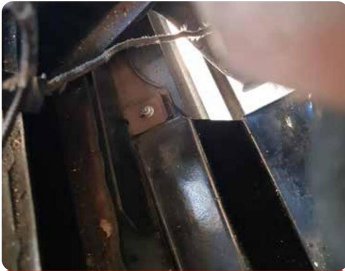
Missing engine mount cover plate
