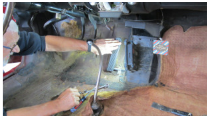
Here is the pesky gas pedal. We needed to remove it to get accurate measurements for the new carpet.
