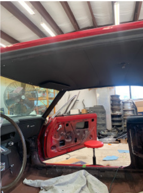
Here the new headliner has been installed. Looks good. page 6
