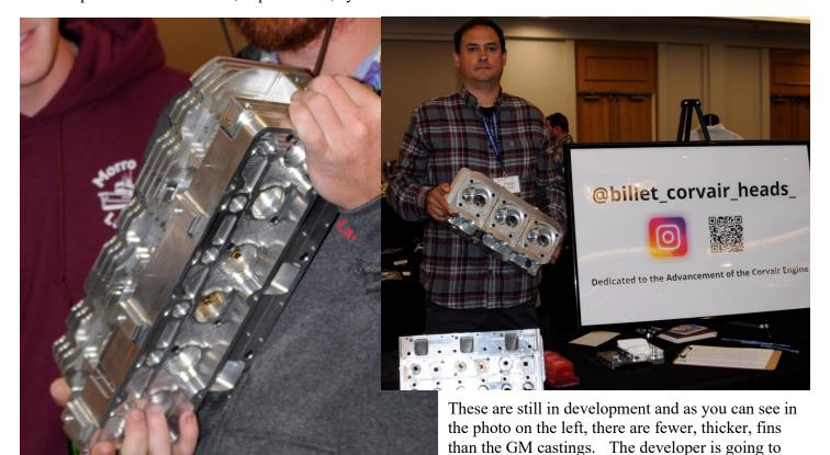
install a set on an engine in the near future and instrument them to see just how well the cooling works. But there's considerable promise here with easily customizable intake manifolds, more modern
