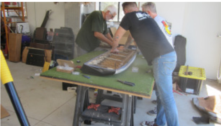
Installing the new rear seat cover is a group effort. Here Don and Josh are holding the new covering material while Ray is applying the hog rings.
