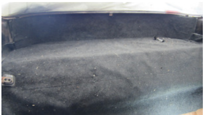
Here the carpeting has been applied to new Package Tray cardboard from Clark's. Spray adhesive was been used. What you don't see is the deadening material that was added first to soften the engine noise.
