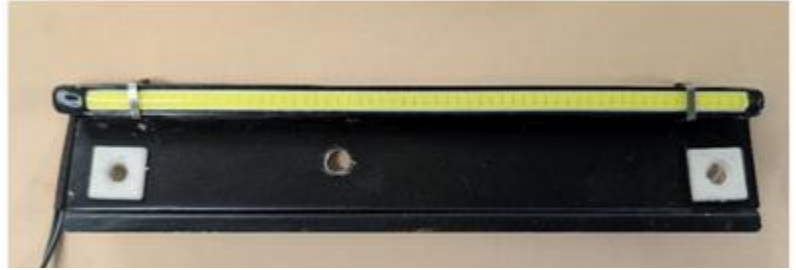
Strip LED light mounted to bracket that attaches to the license plate
