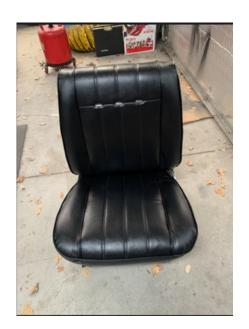
than mine! To recover them you need to remove the emblems so they can be transferred to the new Clark's seat covers. The seat foam was also deteriorat-
