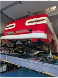
lowered the whole vehicle onto the motorcycle jack, undid the engine mounts, and lifted the vehicle up to leave the powertrain on the jack, which could then be maneuvered into a comfortable position to install the 'new'
